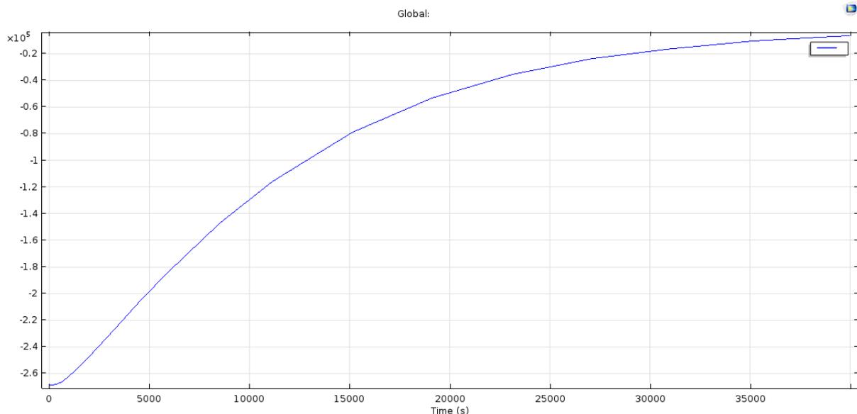
**Figure 2 – The heating phase of the cycle is simulated in order to predict the thermal dynamics of the sleeve/reactor assembly. The curve shows the resulting power input (in Watts: note the 1e5 scale, so the numbers actually show negative power input in units of 100 kW) computed from the controlled temperature at the inlet and the computed water temperature at the outlet, thereby yielding the power requirement for the heating boiler.**
