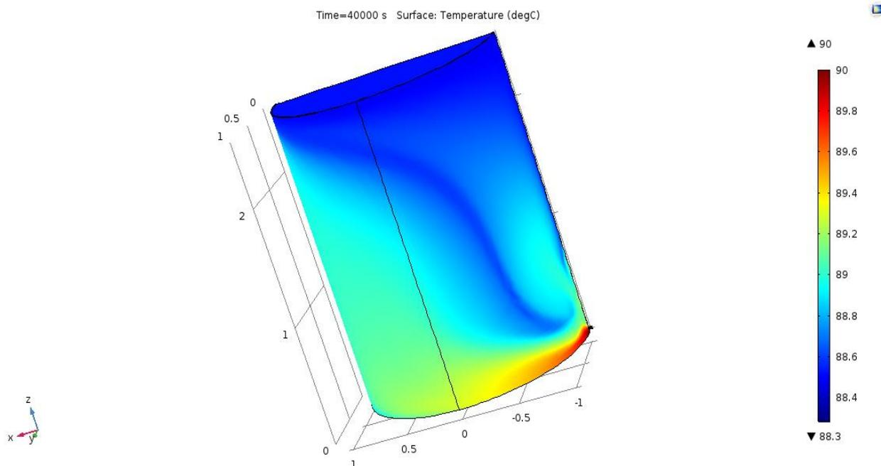
Figure 1 - The heating/cooling sleeve around the reactor is thin. The image shows the surface temperature (in degrees Celsius) of the fluid at the end of the heating phase of the thermal cycle (scale colormap). The swirling flow from the bottom right inlet to the upper left outlet is clearly visible.
